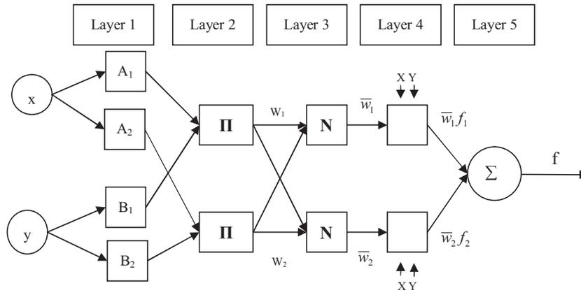
Fig. 1. The architecture of the ANFIS network.
