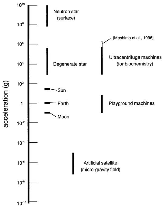
Fig. 1. Acceleration fields that exist in nature or are artificially generated.
