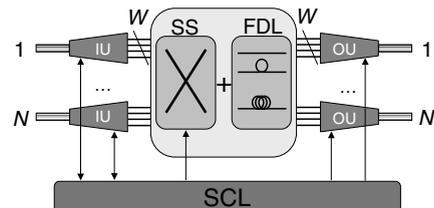
Fig. 1. Generic architecture of a WDM all-optical packet switch with FDL buffer.
