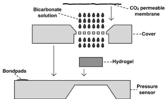
Fig. 1. Schematic representation of the hydrogel-based  $P_{\text{CO}_2}$  sensor.
