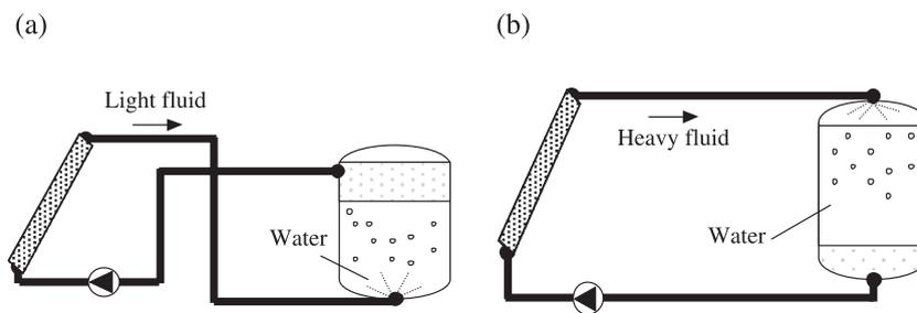
Fig. 1. Schematic diagram of the experimental setup. (a) A working fluid injected into a lighter fluid. (b) A working fluid dispersed in a heavier fluid.
