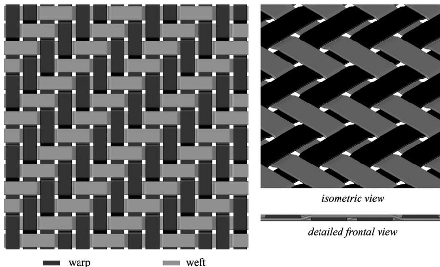
Fig. 1. Model of 2/2-twill weave of the glass-polypropylene hybrid yarn.
