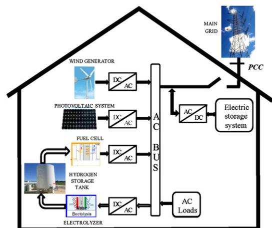
Fig. 1. ZEB-H<sub>2</sub> facility schematic distribution.
