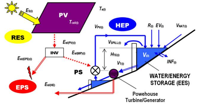
Fig. 2. Operation concept of hybrid solar hydroelectric plant (PV-HEP).
