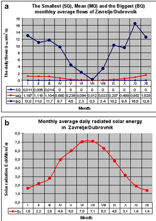
Fig. 1. Hybrid concept with main input resources: (a) Monthly average daily flows (m<sup>3</sup>/s) of the Zavrelje spring [5] and (b) solar radiation at location Zavrelje/Dubrovnik, Croatia [6].
