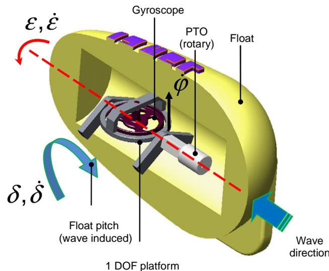
Fig. 2. Gyroscopic mechanism.
