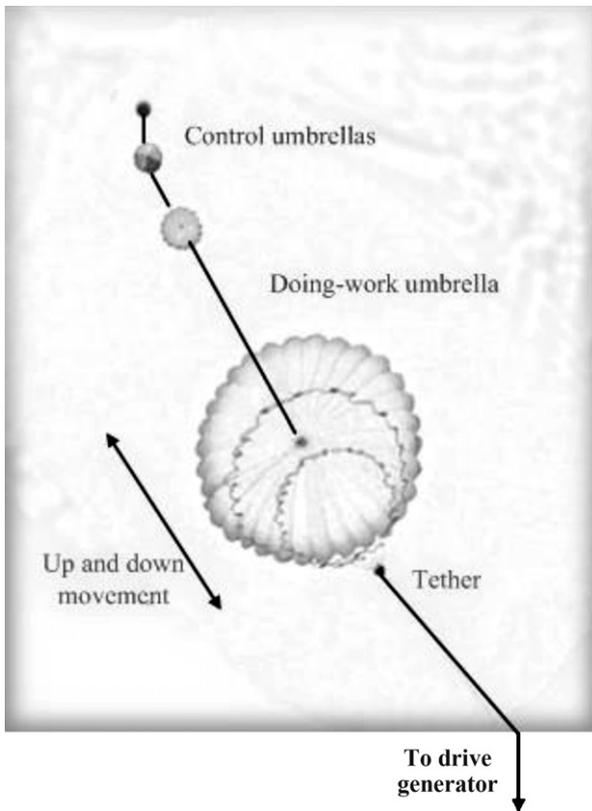
**Fig. 1.** The structure and working principle of the umbrella-ladder combination system.
