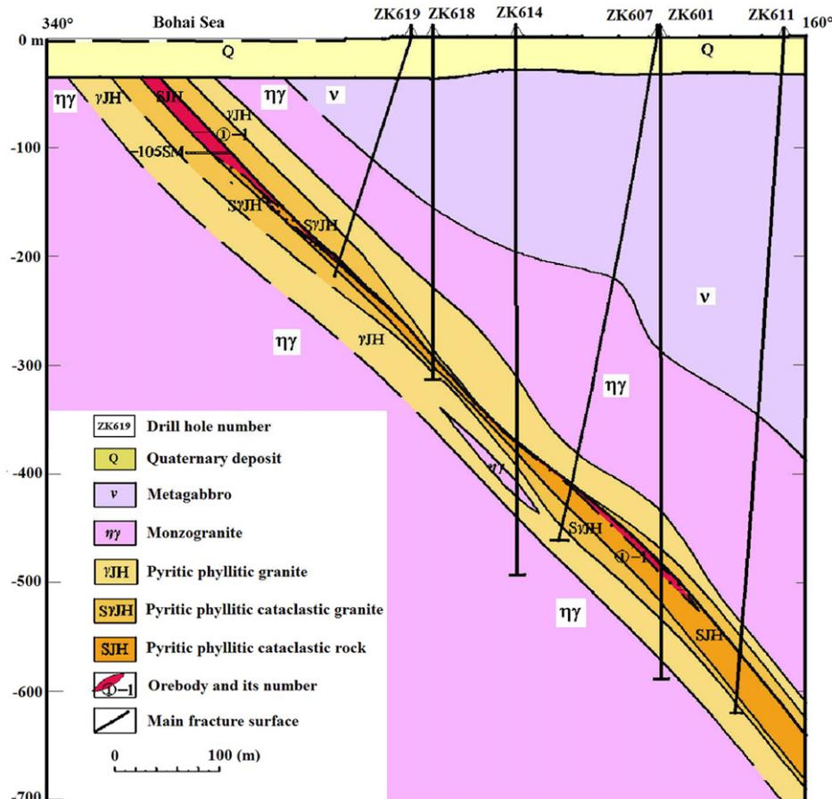
Fig. 1. The geological profile of Xinli Zone at Sanshandao gold mine along the 31# exploration line.
