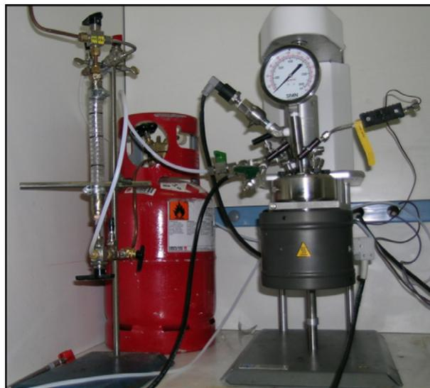
Fig. 1. Experimental set-up for catalytic etherification of glycerol.
