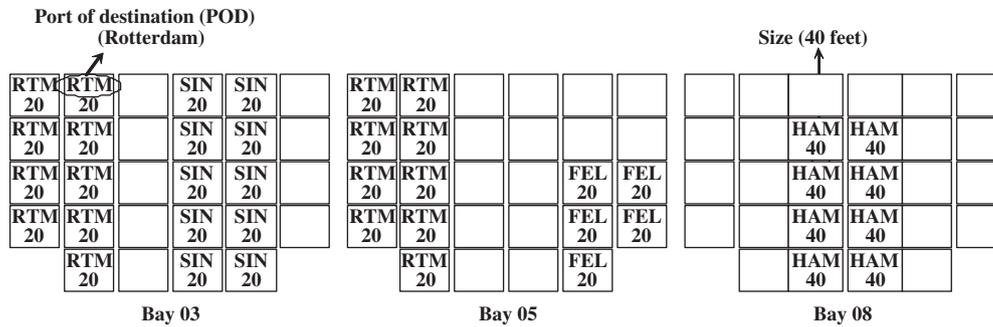
Fig. 1. An example of a stowage plan for a container-ship.
