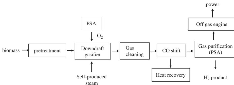
Fig. 2. Process flow diagram of hydrogen production system.
