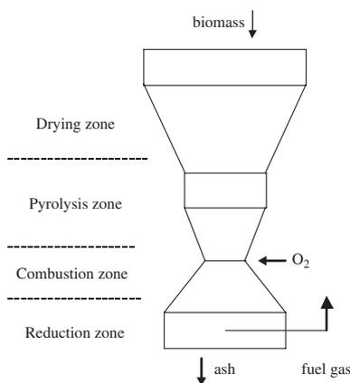
Fig. 1. Schematic diagram of biomass gasification in a downdraft gasifier.
