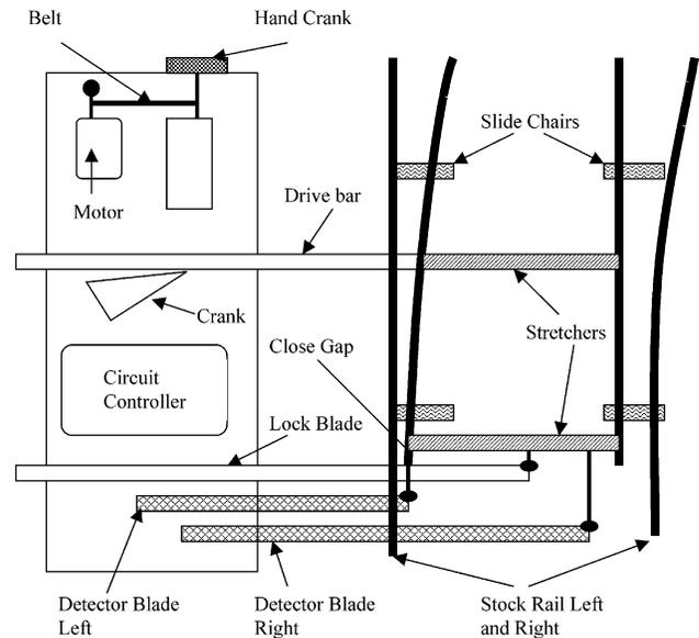
Fig. 1. Point mechanism.
