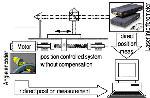
Fig. 1. Measurement setup.
