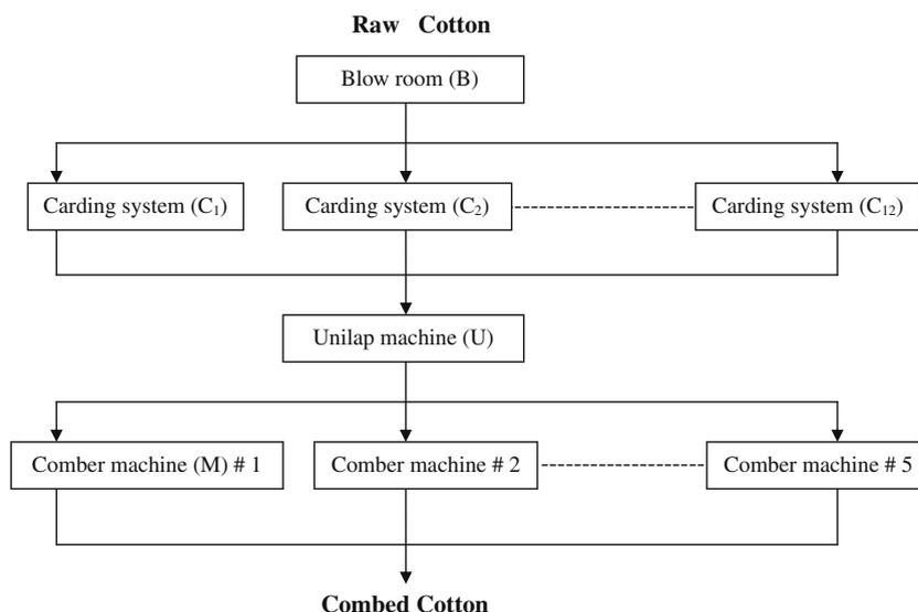
Fig. 1. Flow diagram of combed sliver production system.
