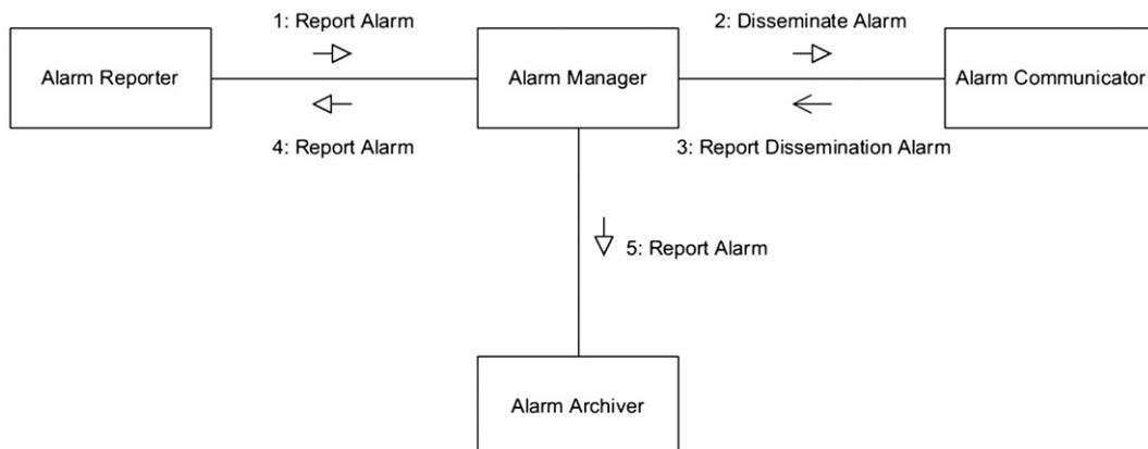
Fig. 1. UML communication diagram of the ACM profile: actors and transactions.
