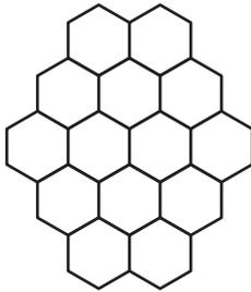
Fig. 1. Cellular structure of a GSM network.
