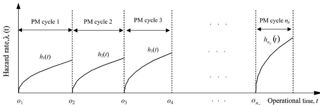
Fig. 1. Hazard rates of PM cycles for the system subject to degradation ( $h_i(t)$  is hazard rate function in the PM cycle  $i$ ;  $o_i$  is start point of the PM cycle  $i$ ;  $i = 1, 2, \dots, n_p$ , and  $n_p$  is number of PM cycles for the system in life cycle).
