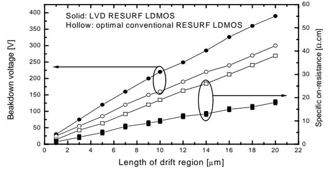
Fig. 3. Trade-off between the breakdown voltage BV and specific on-resistance  $R_{on}$  as a function of the drift region length for the (solid) LVD-RESURF LDMOS and (hollow) conventional optimal RESURF LDMOS.
