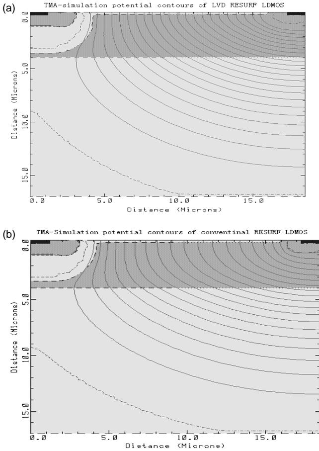
Fig. 1. Simulated potential contours of: (a) proposed LDMOS and (b) conventional RESURF LDMOS with contours = 10 V/step.
