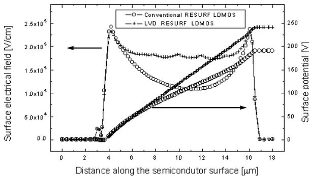
Fig. 2. Surface field and potential distribution of the (O) conventional RESURF LDMOS and (+) LVD-RESURF LDMOS.
