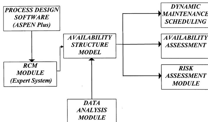
Fig. 1. A proposed industrial equipment reliability management environment.
