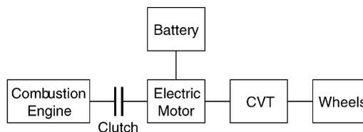
Fig. 1. Block diagram of new PHV configuration.
