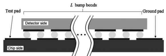
Fig. 1. Scheme of the daisy chain concept.
