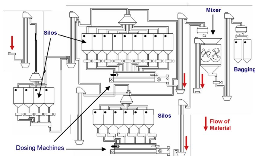
Fig. 1. Production process of Anifeed's food supplements.
