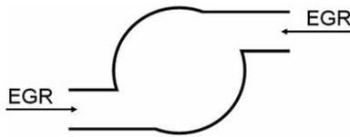
Fig. 1. Axial section (with respect to inlet duct) of air-EGR mixer.
