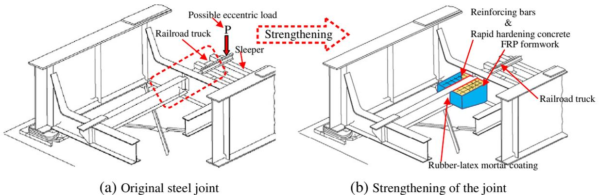
Fig. 1. Images of strengthening of longitudinal and transverse beam connection joint in steel railway bridges.
