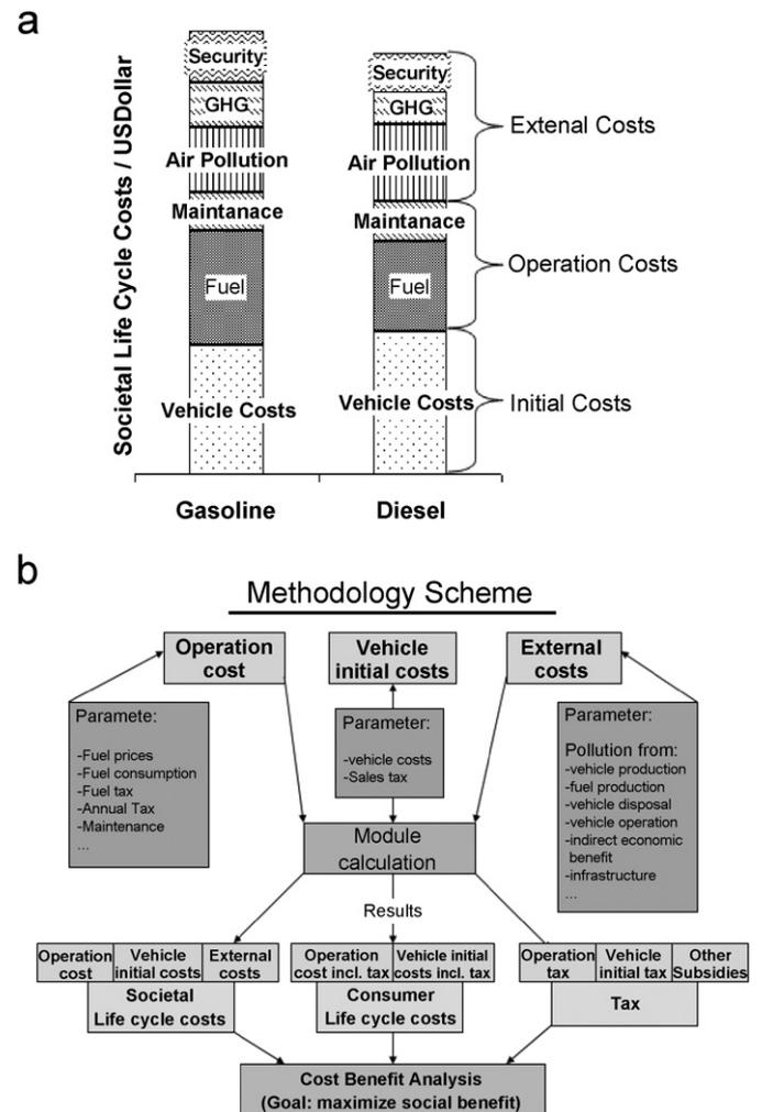
Fig. 1. (a) Example of societal life cycle cost: The sum of initial cost, operation costs and external costs. (b) Scheme for the life cycle cost calculation with cost-benefit-analysis.
