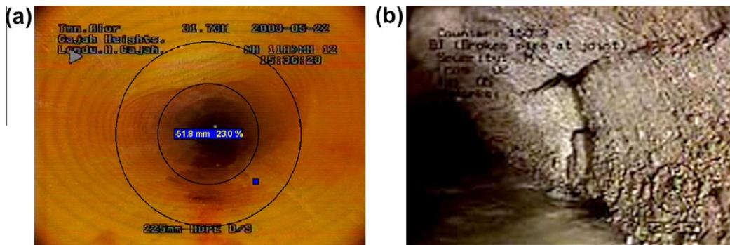
**Fig. 1.** (a) Deformation of DWC-HDPE pipe under external loads, and (b) corrosion of concrete pipe under chemical attack (cases in sewage network captured by CCTV, Malaysia).
