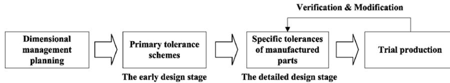
Fig. 1. Flowchart of tolerance design for automotive parts.
