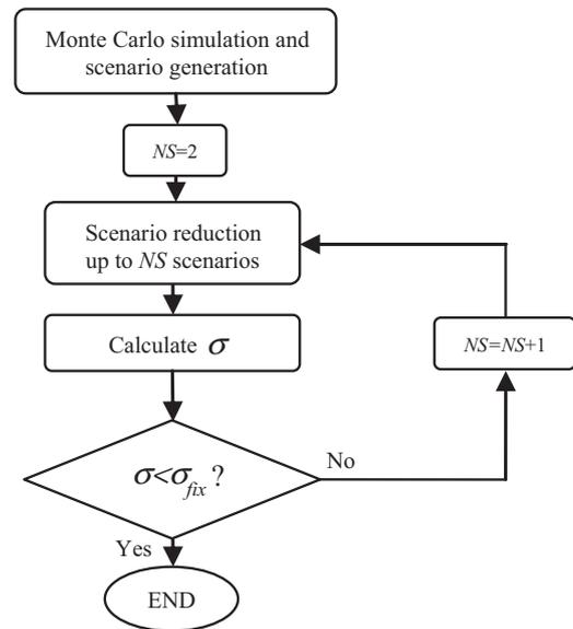
Fig. 1. Flowchart of the scenario reduction algorithm.
