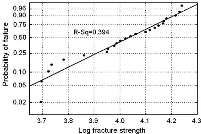
Fig. 1. Linear regression line fitted to the strength data.
