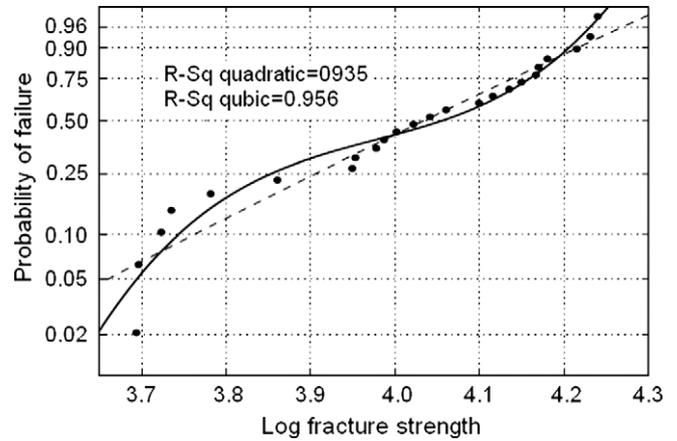
Fig. 2. Curved regression lines fitted to the strength data.
