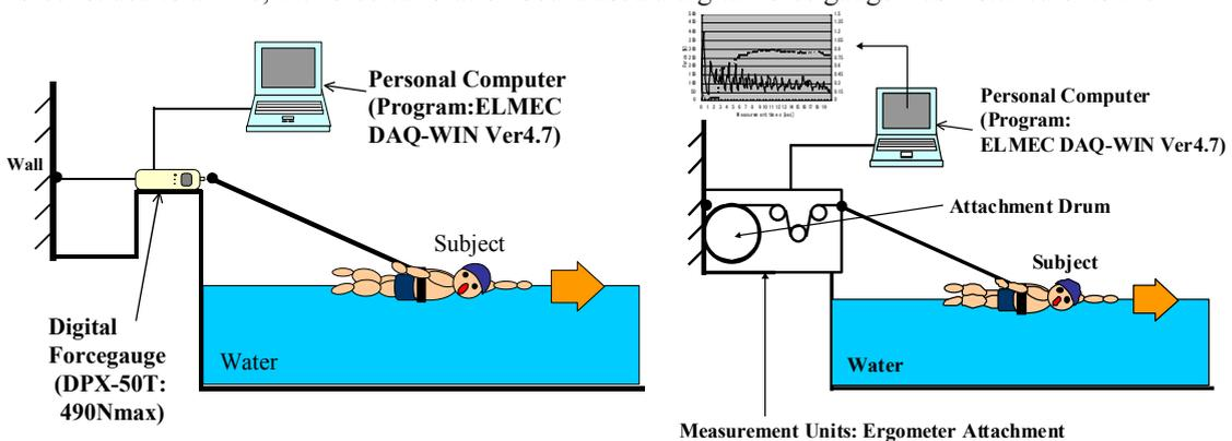
Fig.1. (a) Overview of the force in the TS measurement; (b) Overview of the power in the STS measurement
