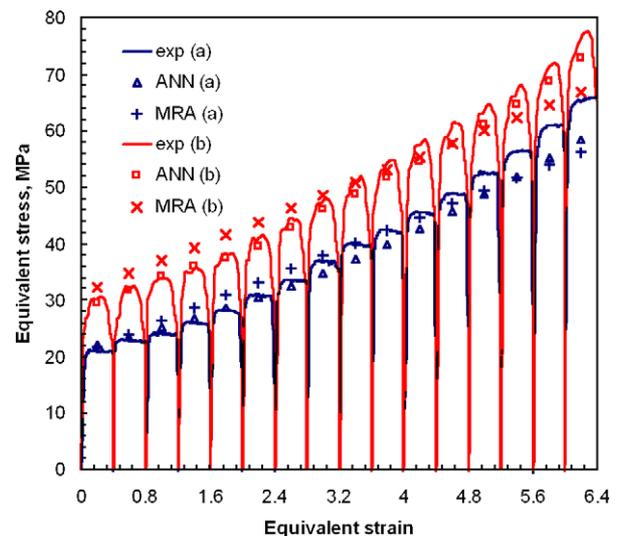
Fig. 1. Effect of strain rate on the experimental flow curve and predicted envelope curves ( $T = 525 \rightarrow 300$  °C;  $t_p = 20$  s;  $\varepsilon_p = 0.4$ ):  $\dot{\varepsilon} = 0.3$  s<sup>-1</sup> (a) and  $\dot{\varepsilon} = 3$  s<sup>-1</sup> (b).
