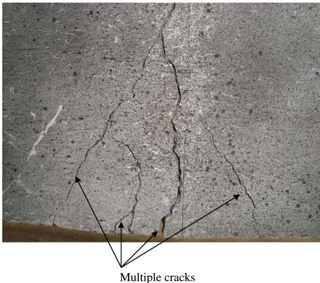
Fig. 1. Multiple cracks developed in RC beam under bending failure [40].
