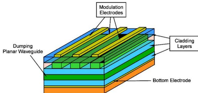
Fig. 1. Schematic structure of the multi-mode waveguide-based EO modulator array.
