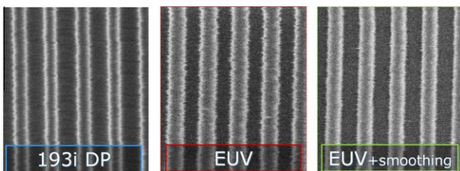
Fig. 1. SEM-CD top-down images of LER affected printed lines.
