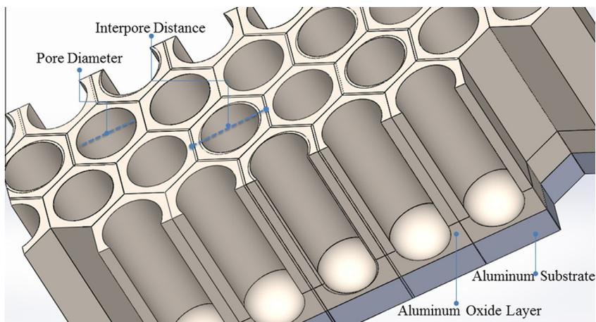
Fig. 1. The schematic geometry of nanoporous anodic aluminum oxide layer and aluminum substrate.
