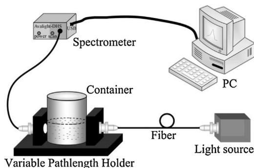
**Fig. 1.** Experimental instrumental setups for UV absorption spectra measurement of the thiophanate-methyl sample solutions.
