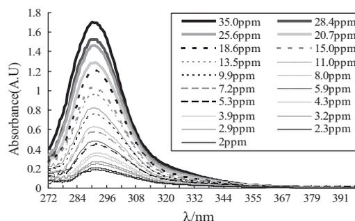
**Fig. 2.** Nineteen samples absorption spectra selected according to statistical analysis method at the different concentrations for establishing model.
