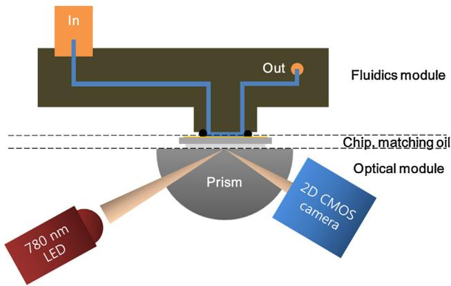
**Fig. 1.** Schematic diagram of a miniaturized SPR biosensor, which consists of flow cells of 2 channels, a 780-nm LED, a cylindrical prism, and a 2D-CMOS image sensor. A gold sensor chip is matched on the prism via immersion oil.
