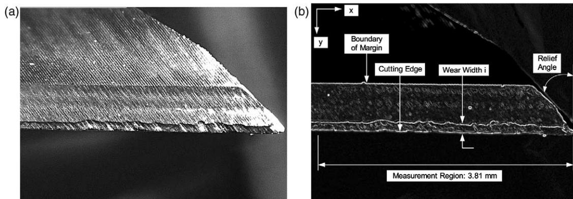
Fig. 2. Preprocessed image of cutting edge (a) and the further processed image showing the wear width and the boundaries (b).
