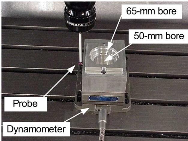
Fig. 1. Spindle touch probe moving to inspect a finished aluminum block mounted on the force dynamometer.
