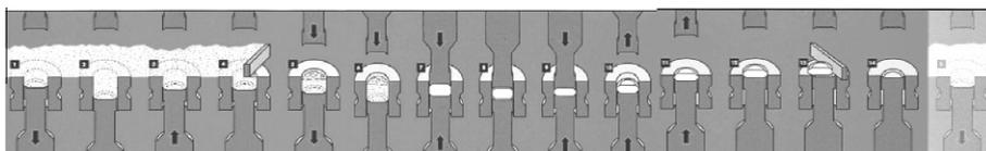
Fig. 2. A schematic illustration of typical production sequence of medical tablets; filling, compression and then ejection stage [2].
