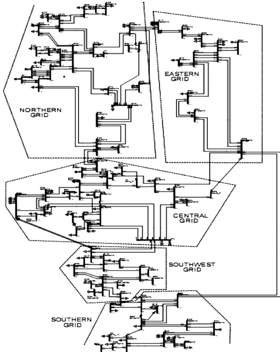
Fig. 2. The 87 bust test system.
