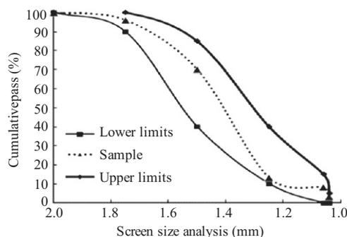
Fig. 1. Screen size analysis for gravel no. 1.
