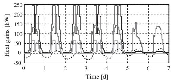
Fig. 2. The various heat gains of the reference building during the first week of July: equipment (black), solar (dark gray), occupants (light gray), and heat loss through building envelope (dotted).
