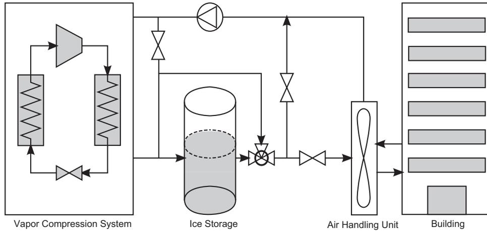
Fig. 1. Cooling system schematics.
