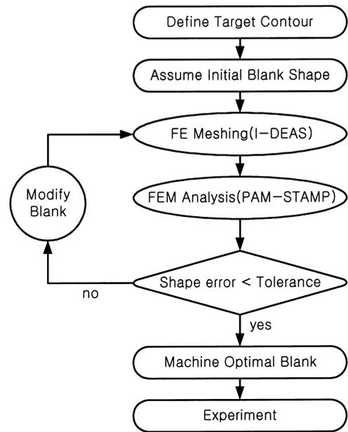
Fig. 3. Flow chart for optimal blank design.
