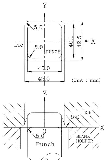
Fig. 4. Die geometry for square cup deep drawing.
