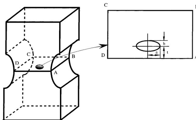
Fig. 1. Three-dimensional planar crack near a free surface.
