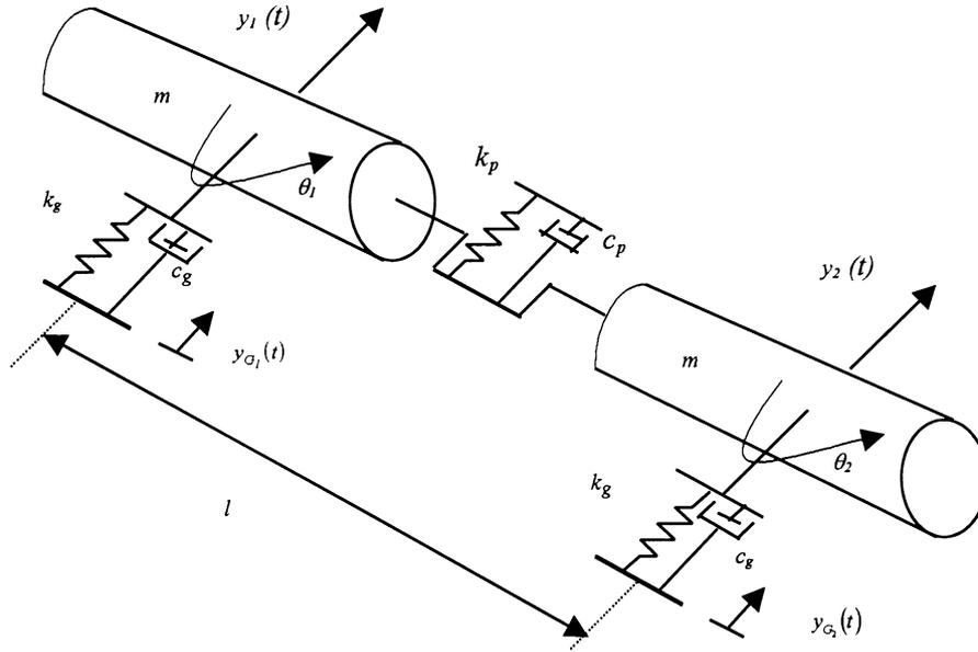
Fig. 1. Idealised structural model for discrete buried pipeline.
