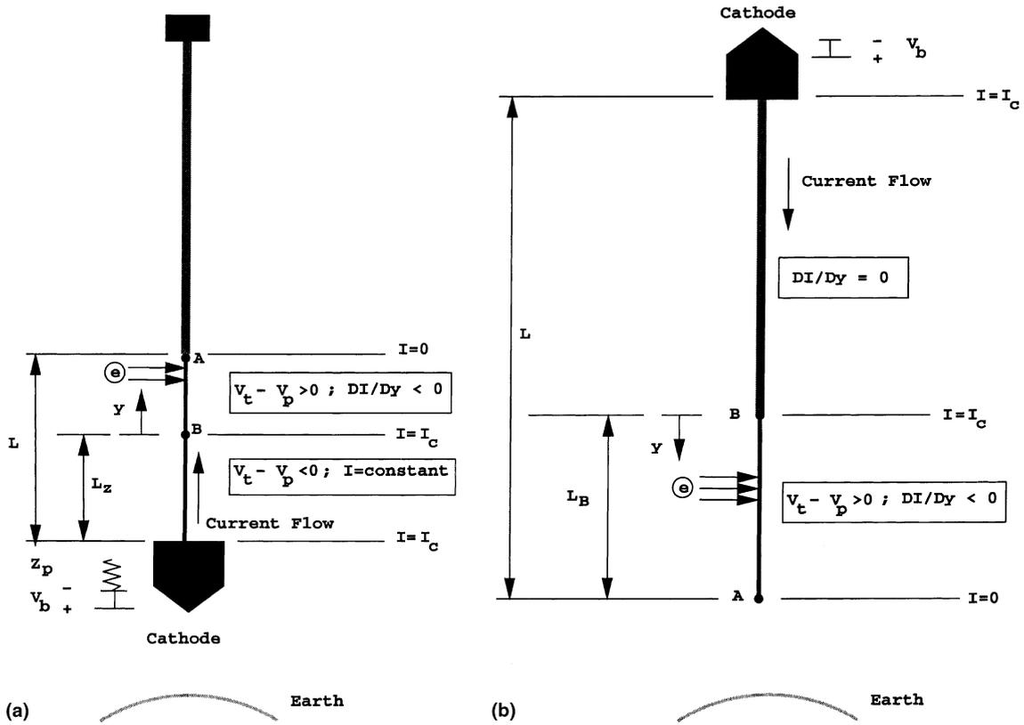
Fig. 1. Generator and thruster configurations of the electrodynamic bare-wire tether: (a) generator; (b) thruster.
