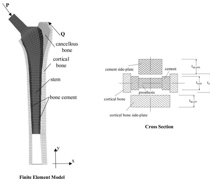
Fig. 1. Finite element mesh and section of the quasi-three-dimensional model of the implant.
